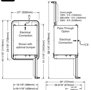
\*33-3/8" (848mm) - with optional 3-1/2" (89mm) casters \*35-1/4" (894mm) - with optional 5" (127mm) casters \*33-3/4" (857mm) - with optional 6" (152mm) legs
