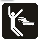
DO NOT OPERATE UNLESS GREASE TROUGH IS INSTALLED.
