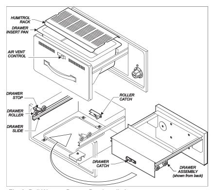
Fig. 8 Roll Warmer Drawer Pan Installation
