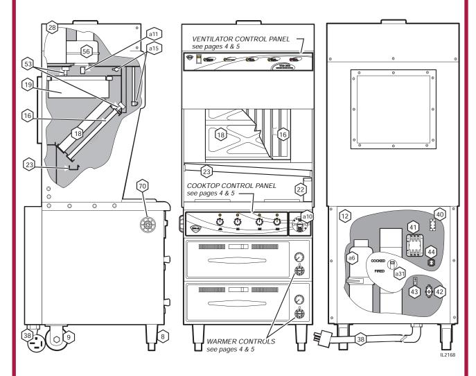
Fig. 1 Ventilator Section Operating Features & Controls
