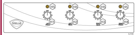
Fig. 3 Cooktop Section Controls & Indicator Lights
