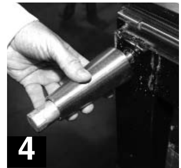
4 Thread leg into cabinet bottom frame rail.
